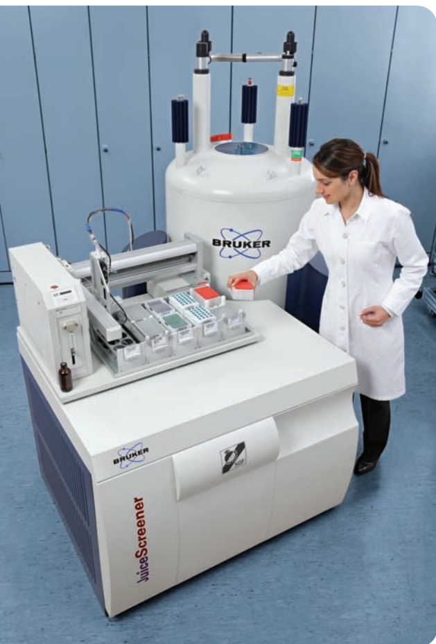
Bruker JuiceScreener™ delivering push-button NMR based quality control of fruit juices.
