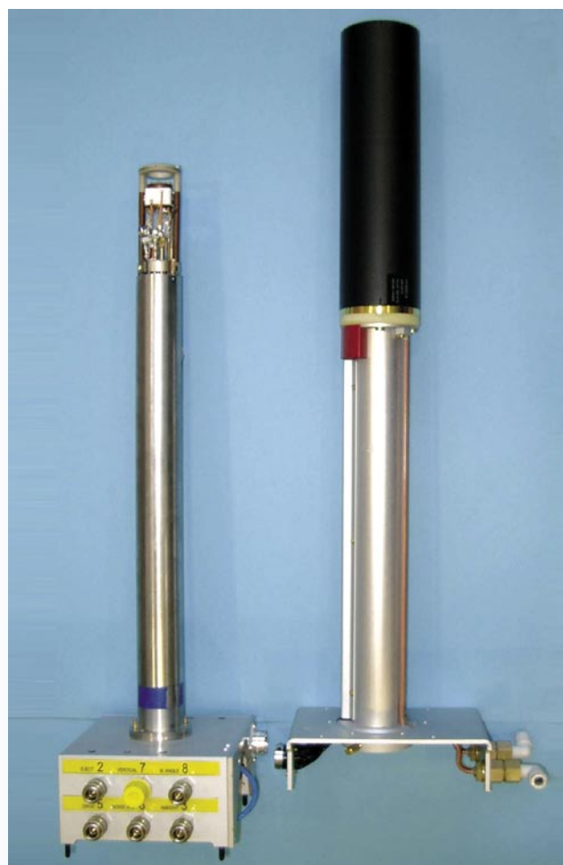
Fig. 1: Bruker components for a HR-MAS-PFG system. A conventional standard-bore HR-MAS probe (left) is inserted into a conventional XYZ gradient system (right) as used for NMR microscopy (Micro2.5, 40 mm i.d.), providing 25 mT/m (2.5 G/cm) per ampere of current.
